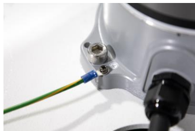
Figure 17: Grounding position for the robot
