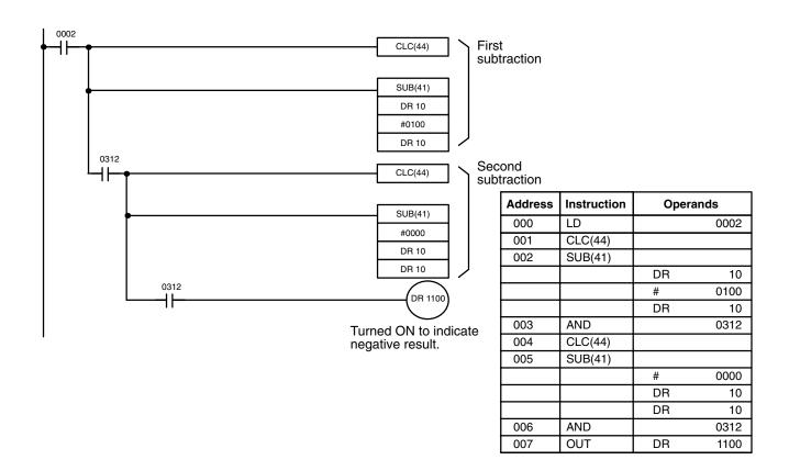
The first and second subtractions for this diagram are shown below using example data for DR 10.
