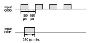
Inputs 0000 and 0001 can be used as normal inputs when CNTH(24) is not used, but the input signals must be 1 kHz max. (500  $\mu$ s wide min.).
