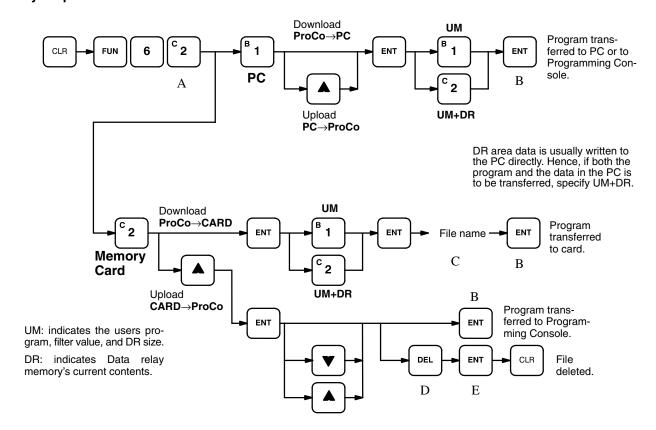
The Programming Consoles displays at different stages of the keying sequence are shown below.
