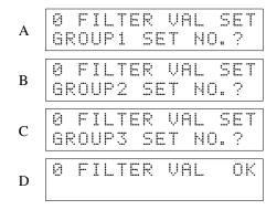
Set the filter values of groups 1, 2, and 3 at the same time. After entering the filter values, read them on the Programming Console for confirmation. Use the following key sequence. Reading is possible in either RUN or PROGRAM mode.
