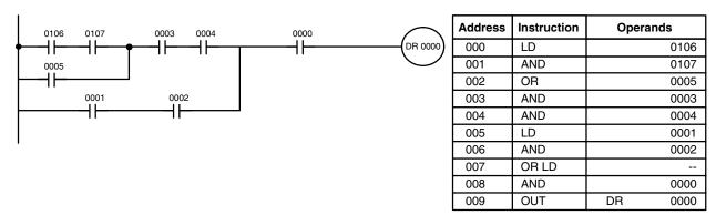
The next and final example may at first appear very complicated but can be coded using only two logic block instructions. The diagram appears as follows:
