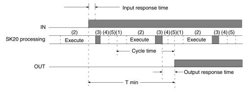
Minimum response time = Input response time + Filter value + Cycle time + Output response time
