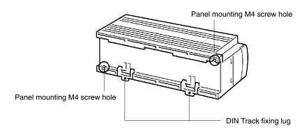
**Note** Install the SK20 such that the heat radiation from top of the unit is not restricted.
