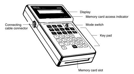
The Programming Console is used to write and transfer programs to the PC. It is also used to monitor operation and modify data. The Programming Console can be connected directly to the PC for single PCs. It can also be connected to other Units via a SYSMAC BUS Remote I/O Unit to access each PC individually without re-connection.
