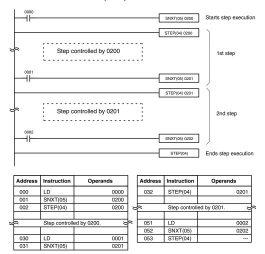
Steps can be programmed in consecutively. Each step must start with STEP(04) and generally ends with SNXT(05). When steps are programmed in series, three types of execution are possible: sequential, branching, or parallel. The execution conditions for, and the positioning of, SNXT(05) determine how the steps are executed.
