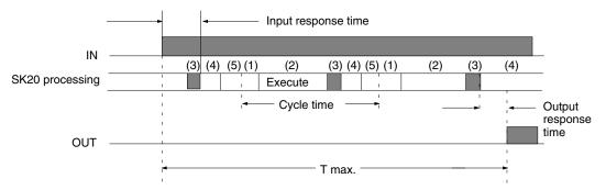
Maximum response time = Input response time + Filter value + (Cycle time x 2) + Output response time
