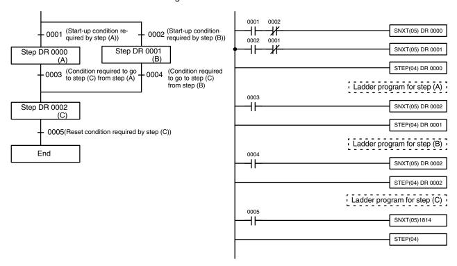
The upper-right program is used if steps (A) and (B) cannot be executed simultaneously. If steps (A) and (B) can be executed simultaneously, delete 0002 (LD NOT) and 0001 (LD NOT).
