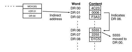
When using indirect addressing, the address of the desired word must be in BCD and it must specify a word within the DR area. In the above example, the content of \*DR 00 would have to be in BCD and between 0000 and 0015.
