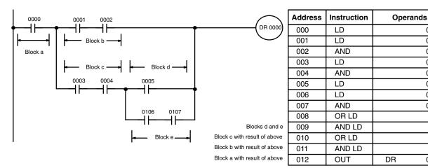
Again, this diagram can be redrawn as follows to simplify program structure and coding and to save memory space.
