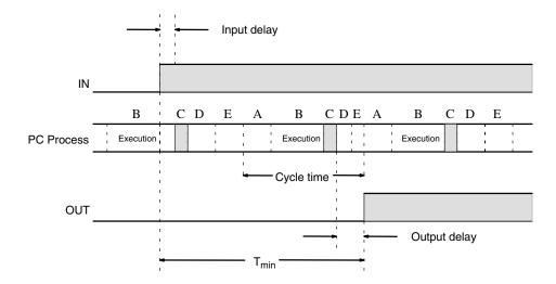
$T_{min}$  = Minimum I/O response time
