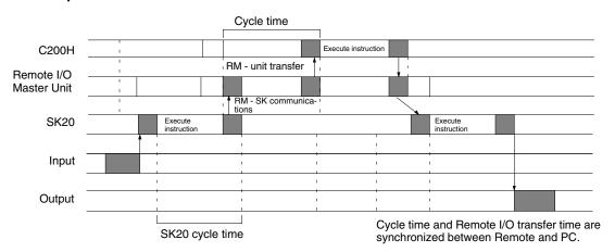
If C200H cycle time exceeds SYSMAC BUS transfer time
