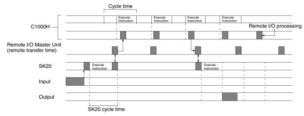
Minimum response time = (C1000H cycle time x 2) + T<sub>RM</sub> + Output ON response time (10 ms) + (SK20 cycle time x 2)
