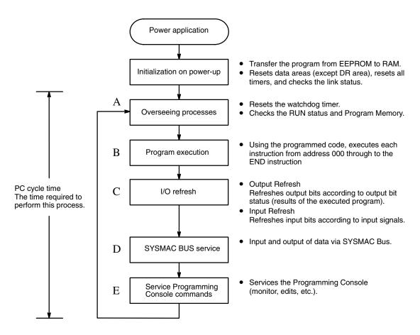
The first initialization process is performed only once, immediately after power is applied to the PC. The remaining operations are performed in cyclic fashion, with each cycle forming one cycle. The cycle time is the time that is
